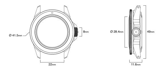
PRODUCT NAMEModello Uno U1S-T-MPTYPESlim Titanium Professional DiverWATER RESISTANCE300m = 1000ft = 30atm WRORIGINMade in ItalyTESTINGSingularly tested for accuracy and water resistanceEDITIONIndividually numbered, edition of 500
